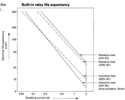
This section explains the derating of the output current of output relays.
