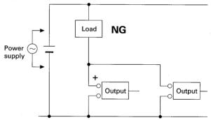
If output relay circuits other than relay contacts are connected in parallel, the leakage current in the OFF state increases. The increase in leakage current adversely affects the connected load.
