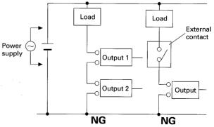
The output circuits must not be connected as shown above.
