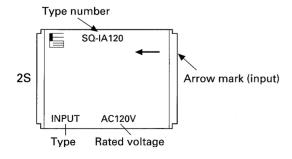
Note: If the top of the case is stained, the top surface must be cleaned with a cloth dipped in lukewarm water. If alcohol is used for cleaning, the markings may be erased.
