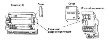
2 Insert each end of the expansion cassette connection cable (NB-EC0005) into each expansion cassette
