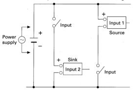
Although the input circuit of a DC input relay has polarity, input relays can be connected in the same circuit with plus input terminals connected to a plus common line, or minus input terminals connected to a minus common line as shown above. This is because the relay input circuits are electrically isolated from each other.
