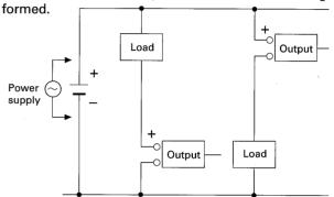
Although the output circuits of DC output relays have polarity, they can be connected as shown above. In another words, output relays can be used as both current sinking output circuit and current sourcing output circuit. This connection is possible because relay output circuits are electrically isolated from each other.
