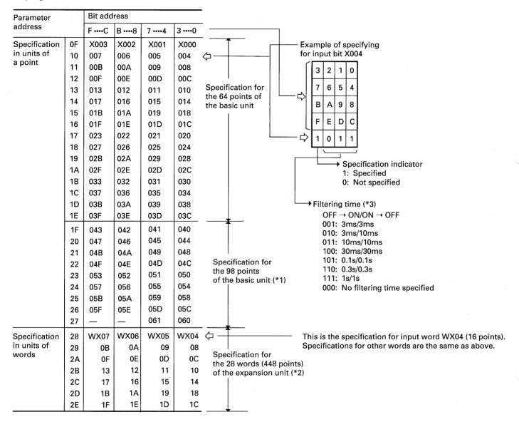
Notes: \*1 If an expansion unit is installed at these I/O addresses (WX04 to WX06), parameter specification (addresses 1F to 27) in units of bits is ignored.
