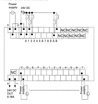
Note: When a DC power supply is used, the positive power supply terminal is on the left.
