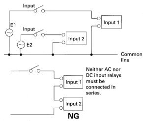
Input circuits must not be connected in series. Voltages E1 and E2 can differ.
