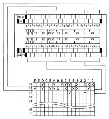
Notes: 1. "X" indicates an input relay and "Y" indicates an output relay.
