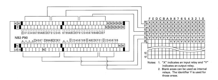
3. I/O address assignment of a system combining the NB1-P40, NB1-E8, and NB2-E56
