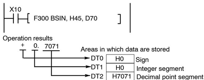
**Example 2: When sending BCD type real-number data stored in “DT0 to DT2”, the F10 (BKMV) block transmission instruction or a similar instruction should be used, and the data sent in three-word units.**
