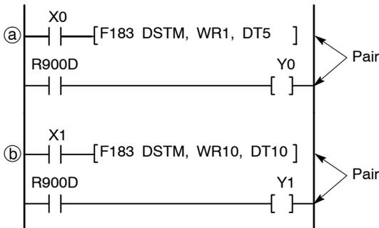
When timer ①, which is activated by X0: on, expires, Y0 goes on. When timer ②, which is activated by X1: on, expires, Y1 goes on.
