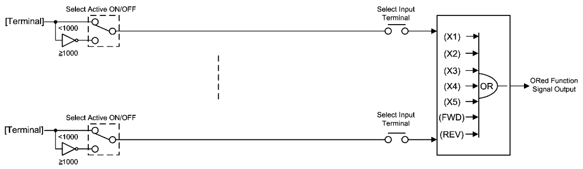
Figure 4.3 (b) Block Diagram of Digital Control Input Block (Only for terminals)
